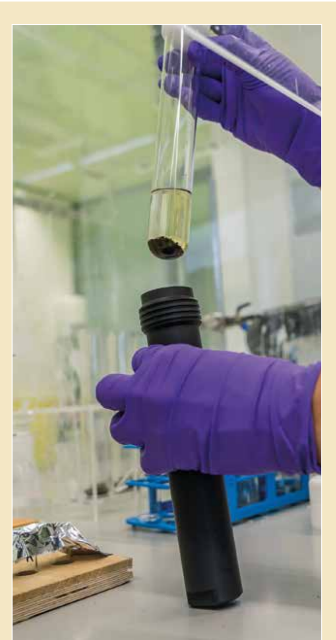
The sediment sample is ground into a fine powder, which is put in a glass tube with a mixture of dichloromethane and methanol. The tube is put in a Teflon-coated vessel and sealed before extraction is begun.
